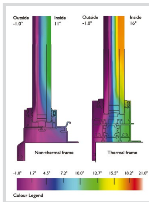
These thermal models show the same outside air temperature but a noticeable difference in the frame temperature on the inside.
